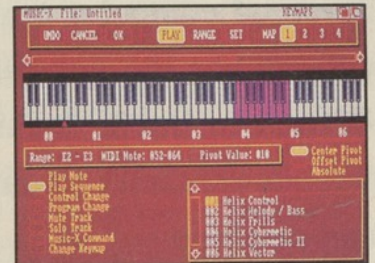
KEYBOARD MAPPING MODULE: Interpret input from your mother keyboard any way you desire, you can even trigger whole sequences from one key. Create up to 128 splits across the keyboard (one for every possible MIDI note).
